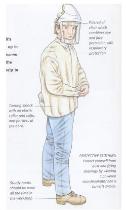
Filtered air visor which combines eye and face protection with respiratory protection. Turning smock . with an elastic collar and cuffs, and pockets at the back.
